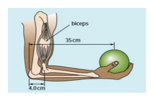
An object of weight 50 N is held in the hand with the forearm at right angles to the upper arm. Use the principle of moments to determine the muscular force F provided by the biceps. Given that the weight of forearm is 15 N, distance of biceps from elbow is 4.0 cm, distance of centre of gravity of forearm from elbow is 16 cm and the distance of object in the hand from elbow is 35 cm
